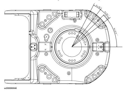
This illustration shows the hole configuration used when securing the robot.
