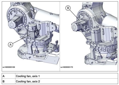
2.3.11 Installation of cooling fan for motors (option) *Continued*
